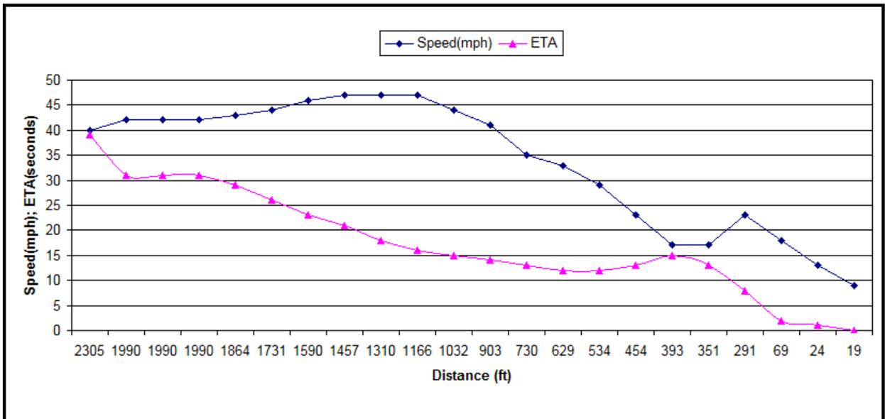
Graphs showing changes in ETA as a result of speed changes during the Tamien station approach
